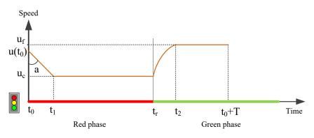
Figure 2: Optimum speed profile in case 2.
